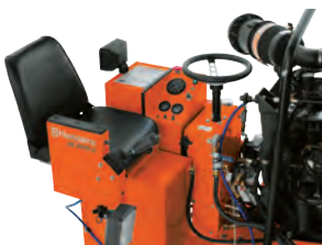
Tilt steering - Tilt steering for increased operator comfort.
